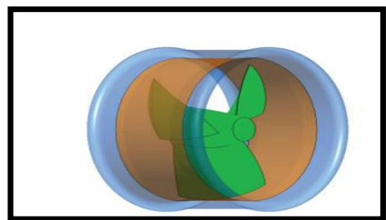
**Fig1:** Wall counter rotate thruster
