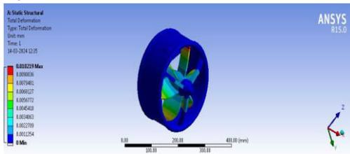
Fig 15: Total deformation of Al 6061 material
