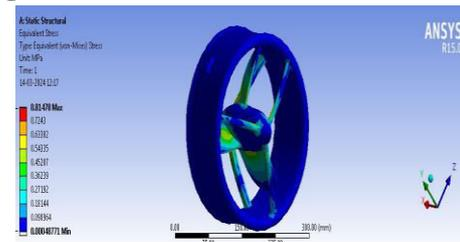
**Fig 8:** Von-misses stress of CFRP material
