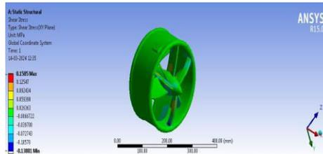
**Fig 11:** Shear stress of Al 6061 material
