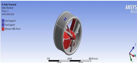
**Fig 6:** Moment 1000 N.mm for 6 propeller
