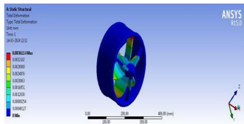
Fig 16: Total deformation of CFRP material
