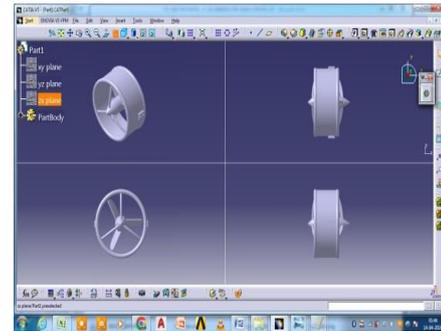
**Fig 2:** Multiple views of thruster
