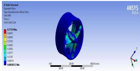
Fig14: Von-misses stress of CFRP material
