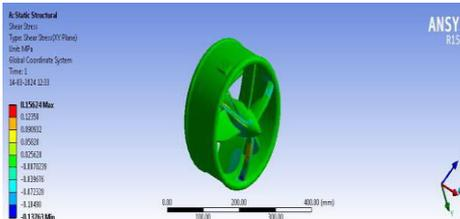
**Fig 12:** Shear stress of CFRP material
