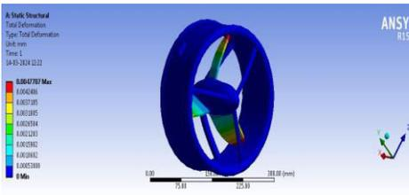
**Fig 10:** Total deformation of CFRP material
