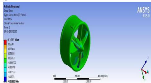
Fig17: Shear stress of Al 6061 material
