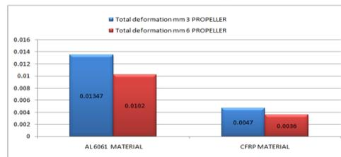
Fig 20: Total Deformation
