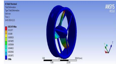
**Fig9:** Total deformation of Al 6061 material
